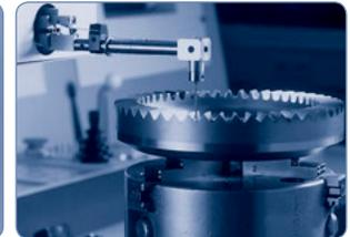
Computerized mapping of gear tooth profile
