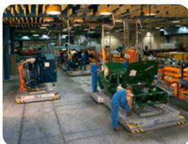
World's first automobile production plant with driverless vehicles
