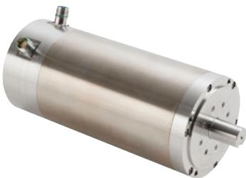
These brushless servo motors incorporate pressure compensation technology to allow underwater operation up to 20,000 ft while withstanding extreme environments. They feature stainless steel and aluminum nickel bronze housings or an anodized aluminum housing for lighter overall weight. All shafts are stainless steel and sealed with an externally serviceable O-ring seal. The S Series is fully tooled for cost-effective volume production.
